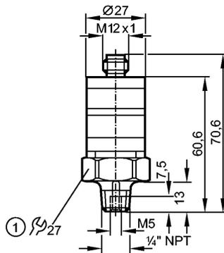
1: tightening torque 25 Nm
